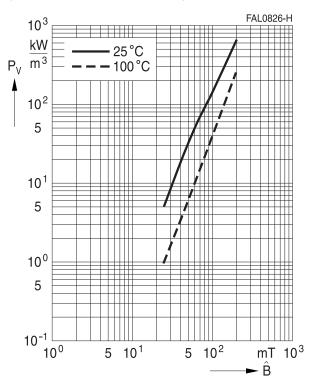
Relative core losses versus temperature (R34 toroids, f = 100 kHz)
