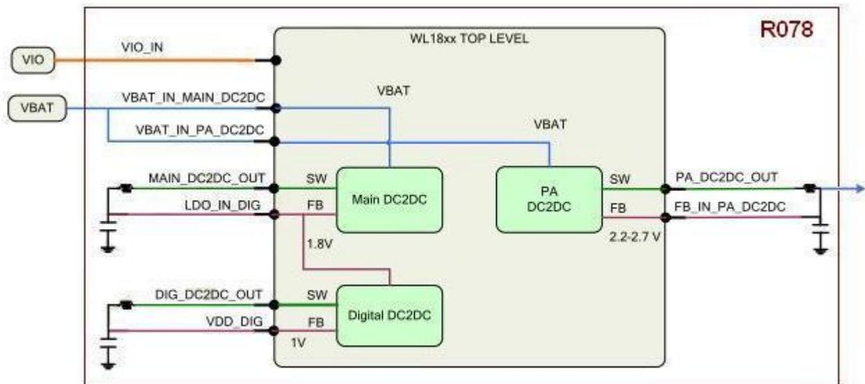
Figure 3-3 Internal DC2DC's
