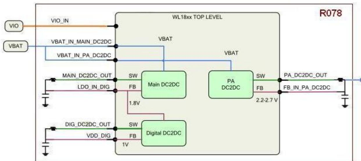
Figure 3-3 Internal DC2DC's
