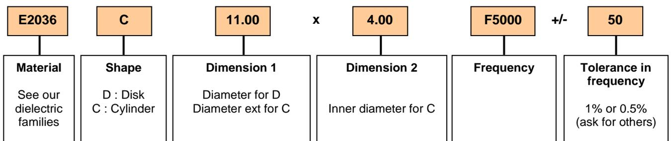
Example for dielectric resonator with spacer in dimension: E2036/AL C 11.00x4.00x5.35
