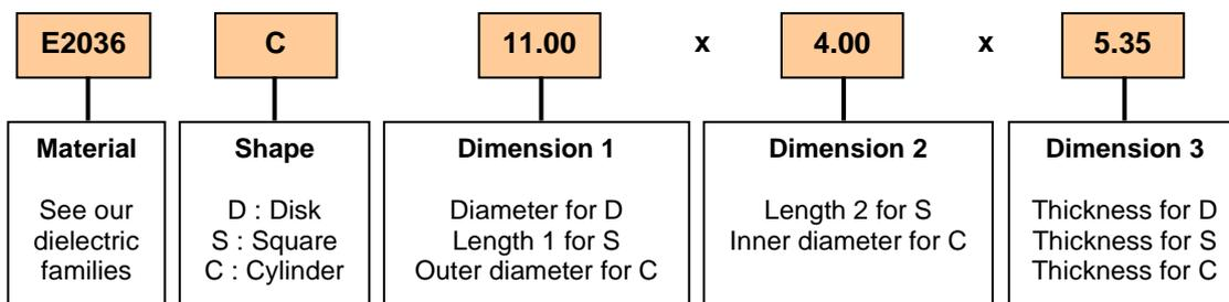
Example for dielectric resonator in frequency: E2036 C 11.00x4.00 F5000+/-50
