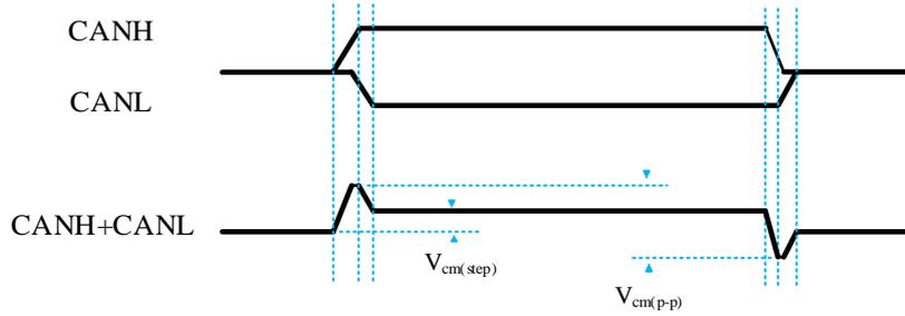
Fig 9 CAN bus common-mode voltage (according to SAE 1939-14)
