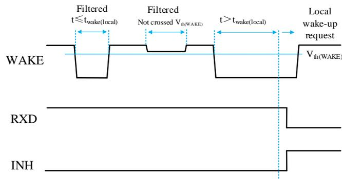
**Fig 4 Local wake-up for WAKE falling edge**
